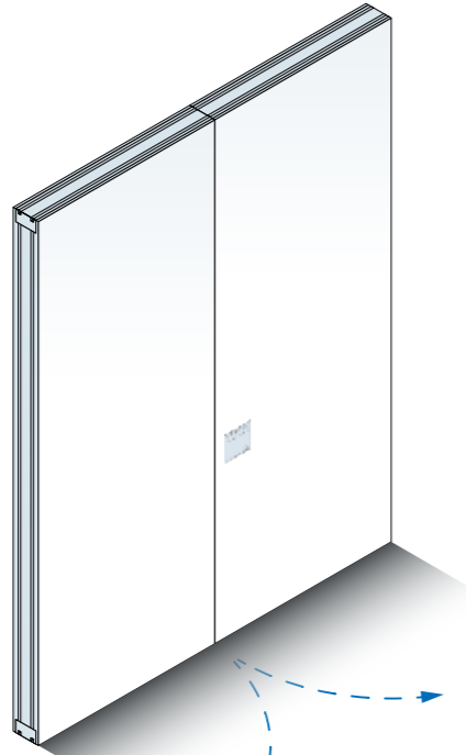
Basic Panel Bi-Parting System With one active pass door and one passive pass door
