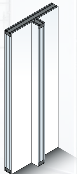
Junction Panel T (JPT)
